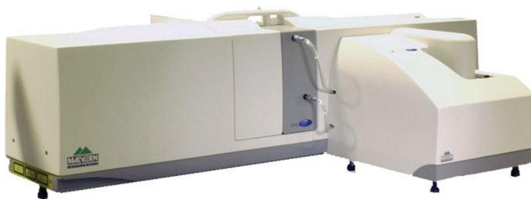
**Figura 11:** Instrumento Mastersizer 2000 Malvern.
