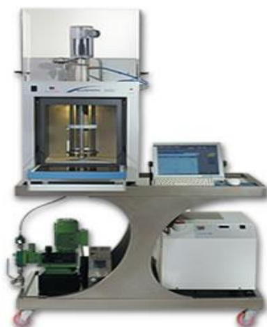
**Figura 14:** Reator micro-ondas multimodo FlowSYNTH Milestone.
